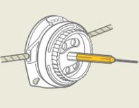
**F** Loosen (but do not remove) set screws, then remove lace.
