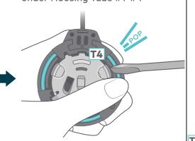
Verify Housing Spring is 13 secure under Tabs #1-#4
