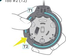
Note: It is helpful to hold Housing Spring between Housing Tab #1 (T1) and Tab #2 (T2)
