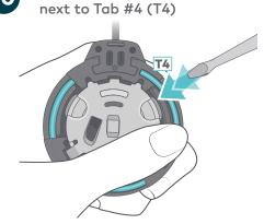
Note: Hold Housing Spring and housing at Tab #3 (T3) location
