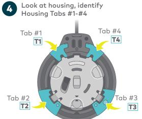
**End of Housing Spring** should contact the Housing Tab #1 (T1)
