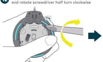
Housing Spring should be secure under Housing Tabs #1-#4
